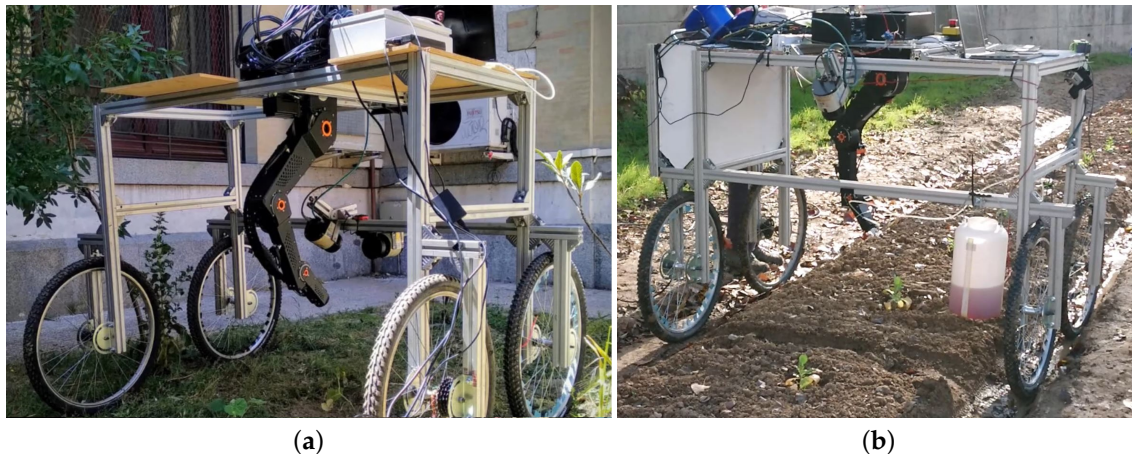
Figure 2. Structure with the robot arm positioned in the center of the platform. (a) mobile platform assembled, (b) robotic platform—on field. Source: Author.
