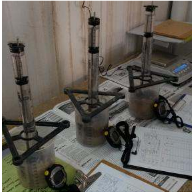
Fig. 3. Mini disk infiltrometer used for laboratory infiltration measurements
