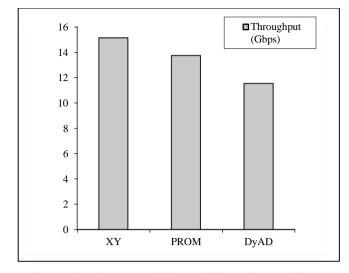
Fig.6. Throughput Analysis graph for routing techniques
