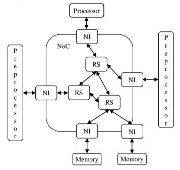
Fig.1. Basic Components of NoC Router
