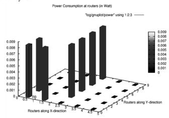
Fig.3. Power Consumption graph for XY routing
