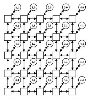
Fig.2. Architecture of  $5 \times 5$  Mesh based Noc
