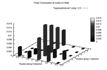
Fig.4. Power Consumption graph for PROM routing
