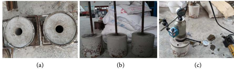
**Figure 2.** Experimental steps. (a) Preparation of test blocks; (b) Anchor rod anchoring; (c) Anchor rod pulling.
