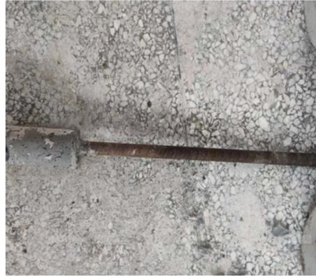
**Figure 8.** Failure state diagram of surrounding rock anchor solid interface.
