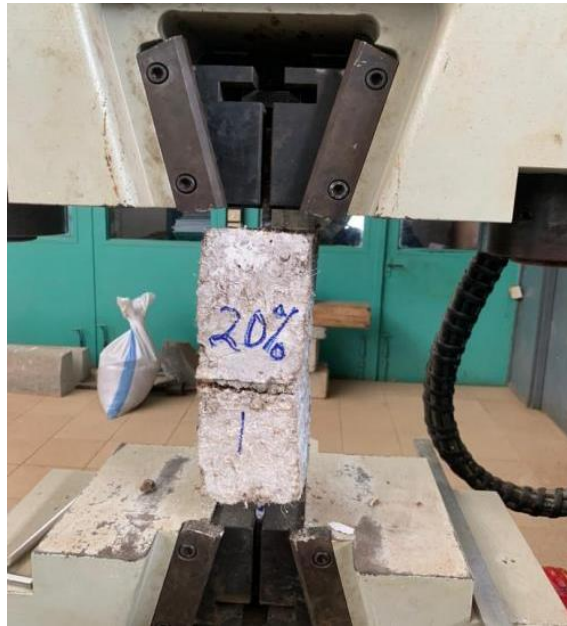
Fig. 7. Bond failure mechanism
