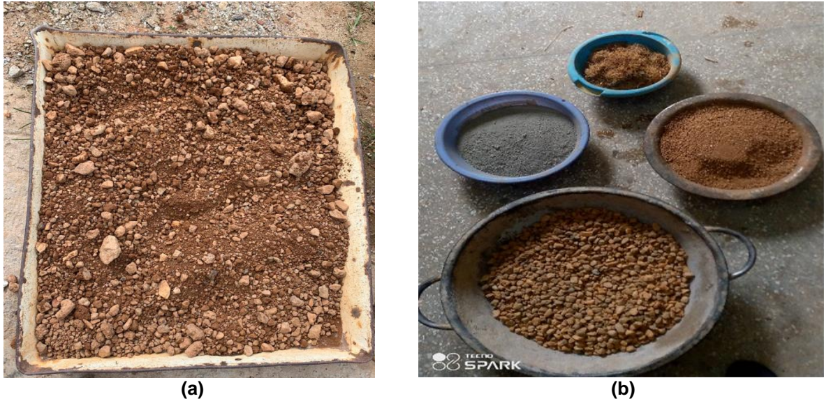
Fig. 1. (a) Laterite soil (b) Cement, Fine aggregates, Coarse aggregates and Palm kernel fibre
