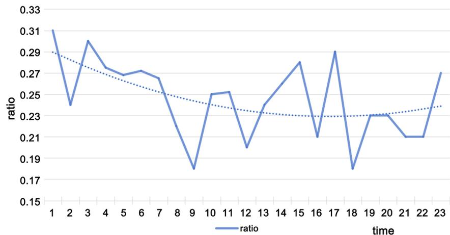
**Figure 8.** The relation of operation hours with the ratio of the condensation heat can be recovered of the experimental in the hotel in south china.
