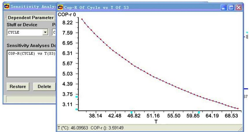
Figure 5. The relation of COP with the temperature of the outlet of the condenser (S3).
