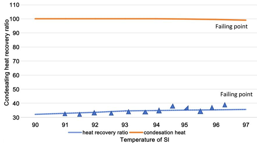
**Figure 7.** Some points of the relation of temperature of outlet of compressor with the ratio of the condensation heat can be recovered.
