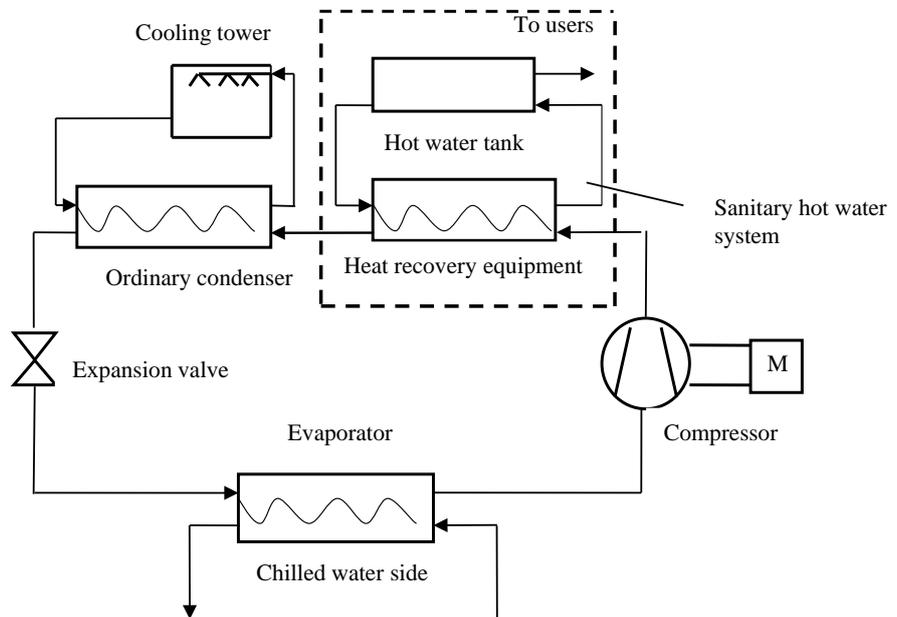
**Figure 1.** Schematics of a vapor-compression refrigeration cycle.
