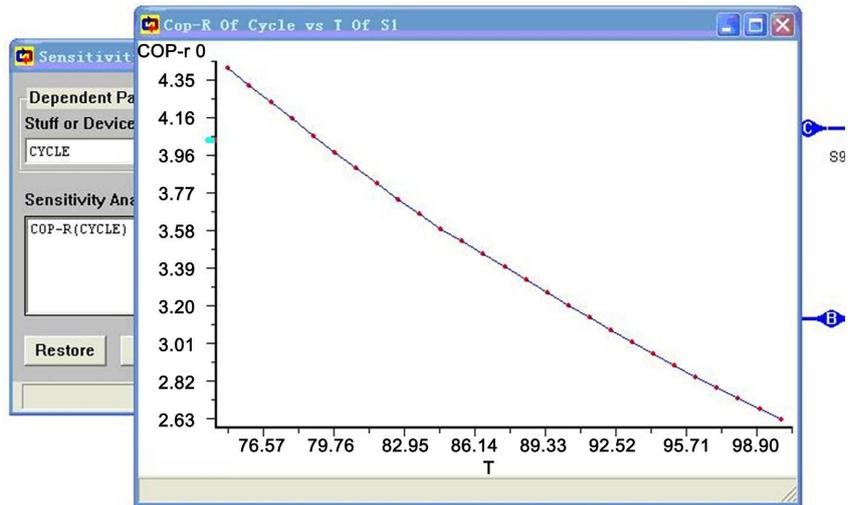
Figure 4. The relation of COP with the temperature of the outlet of compressor (S1).
