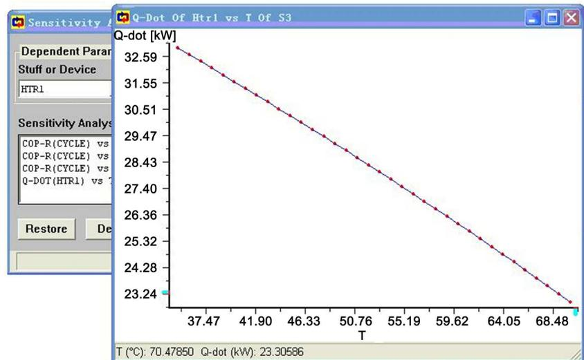
Figure 6. The relation of refrigeration effect with the temperature of outlet of the condenser (S3).
