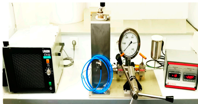
Figure 2. Freeze isostatic pressure equipment at ICMCB.
