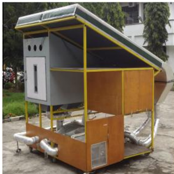
Fig. 8. Solar assisted heat pump dryer (SAHPD)
