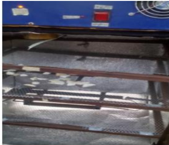
Fig. 10. Hybrid solar dryer coupled with electrical heating element
