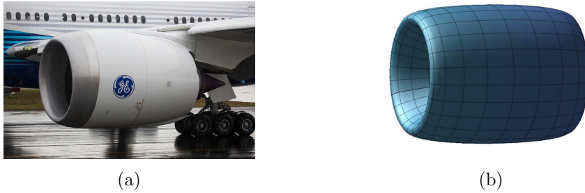
Fig. 1. Comparison of the GE90-115BL Turbofan (shown in Fig. (1a)) [9] on the Boeing 777 Jet and the Spherical Biconcave Disc intended to mimic its shape. The Spherical Biconcave Disc in Fig. (1b) was taken under parameters \rho = 1.963m , A = 0.05 , and B = 0.78 .
