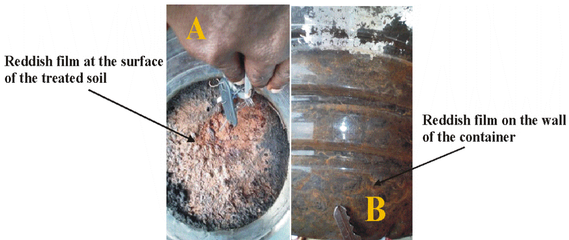
Photograph 3. Presence of a reddish film at the surface of the soil-rock mixture and on the walls of the container
