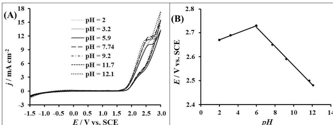
Fig. 9. (A) Cyclic voltammograms recorded on BDD at different pH in H<sub>2</sub>SO<sub>4</sub> (0.1 M) containing 3.2 mM of IOX at 50 mV s<sup>-1</sup>; (B) Peak potential as a function of pH
