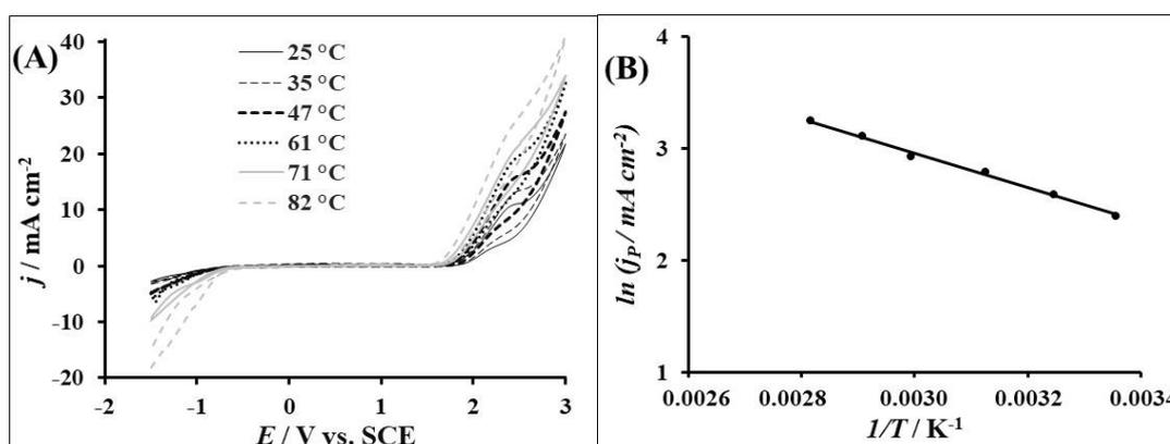
Fig. 4. A) Cyclic voltammetry curves recorded on BDD electrode at several temperatures in 0.1 M H<sub>2</sub>SO<sub>4</sub> containing 3,2 mM IOX under the potential scan rate: 50 mV s<sup>-1</sup>, (B) plot of ln j<sub>p</sub> = f (1/T)
