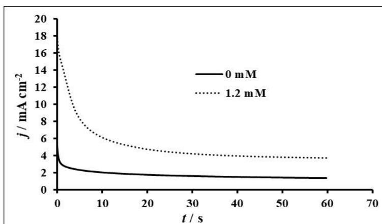
Fig. 10. Chronoamperometric curves in 0.1 M H<sub>2</sub>SO<sub>4</sub> (pH = 9), in the absence and presence of 1.2 mM IOX
