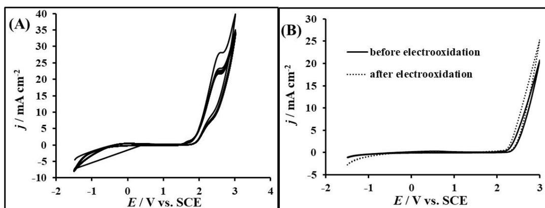
Fig. 3. (A) Cyclic voltammogram of BDD in 0.1 M H<sub>2</sub>SO<sub>4</sub> for 23 successive Cycles in scans performed; (B) Cyclic voltammogram of BDD in 0.1 M H<sub>2</sub>SO<sub>4</sub> before and after electrooxidation
