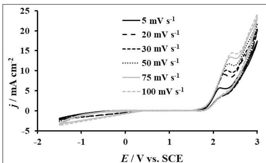
Fig. 5. Cyclic voltammery curves recorded on BDD electrodes in 3,2 mM IOX containing in 0.1 M H<sub>2</sub>SO<sub>4</sub> at several potential scan rates (5-100 mV s<sup>-1</sup>)
