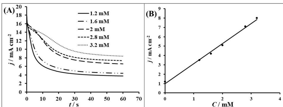
Fig. 11. (A) Chronoamperogram of BDD in H<sub>2</sub>SO<sub>4</sub> (0.1M) pH=9 media with several concentrations of IOX. Applied potential  $E = 2.4$  V vs. SCE; (B) Current density versus IOX concentration curve
