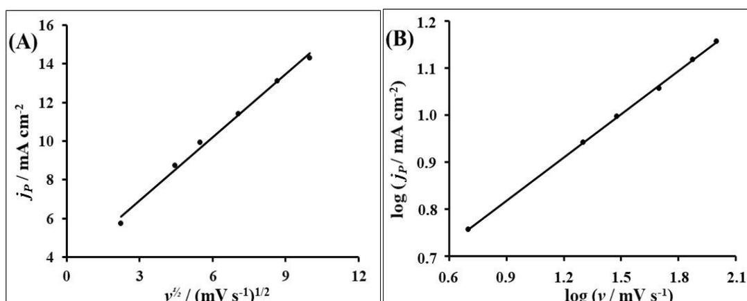
Fig. 6. (A) Evolution of the peak of current density against the square root of the potential scan rates  $j_p$  vs.  $\nu^{1/2}$ . (B); Plot of log  $j_p$  vs. log  $\nu$
