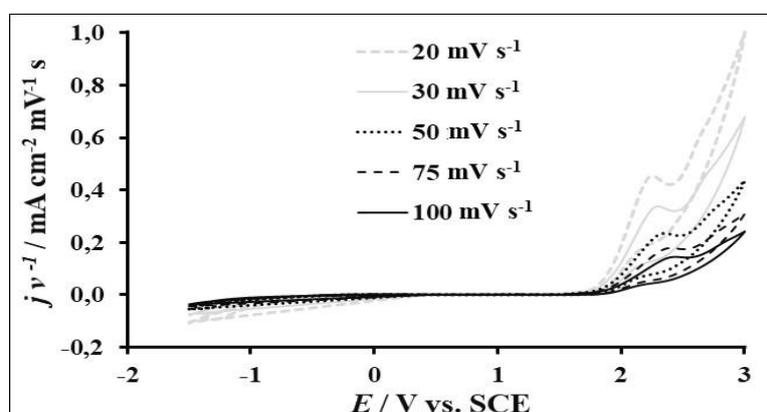
Fig. 8. Normalized current density of the cyclic voltammety measurement recorded on BDD in  $0.1 \text{ M H}_2\text{SO}_4$  containing  $3,2 \text{ mM IOX}$  with the potential scan rates ( $20\text{-}100 \text{ mV s}^{-1}$ ) versus applied potential
