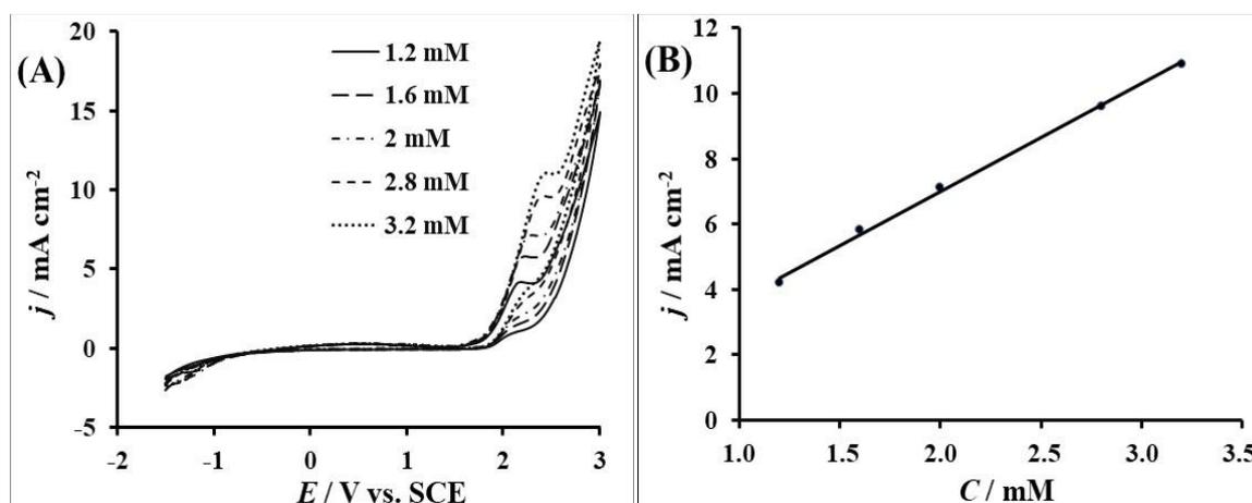
Fig. 2. (A) Cyclic voltammetry curves recorded on the BDD in  $\text{H}_2\text{SO}_4$  (0.1M) in the presence of different IOX concentrations at  $50 \text{ mV s}^{-1}$ ; (B) plot of current density of the IOX oxidation peak versus IOX concentrations
