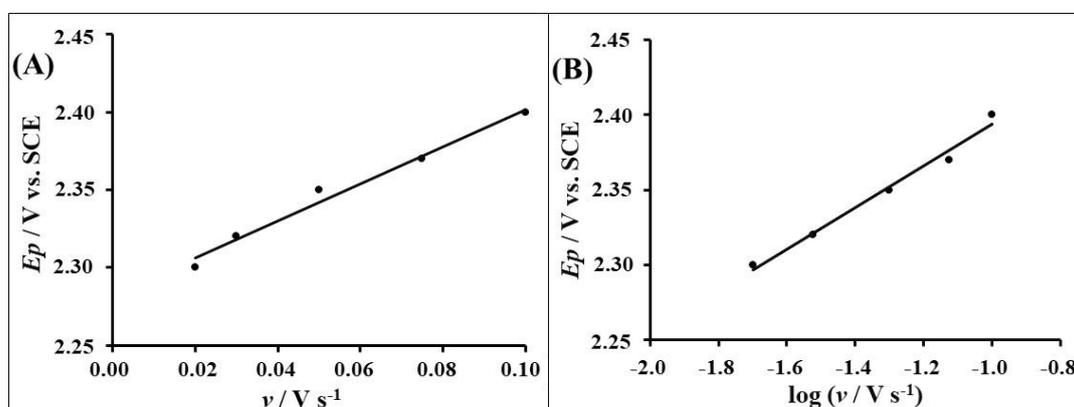
Fig. 7. (A) Dependence of peak potential ( $E_p$ ) on the potential scan rate ( $v$ ); (B) Variation of the scan rate normalized current with scan rate
