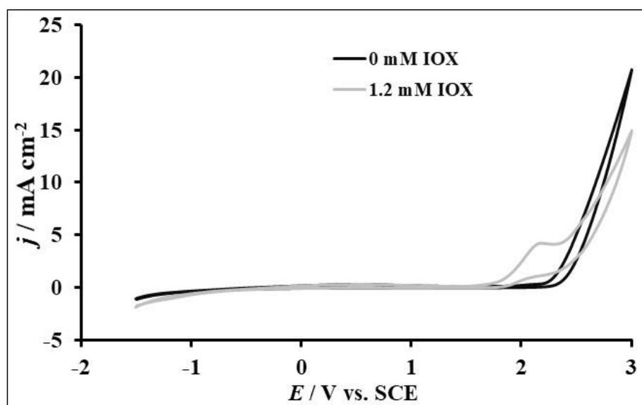
Fig. 1. Cyclic voltammograms of BDD in 0.1 M  $\text{H}_2\text{SO}_4$  in presence and absence of IOX at  $50 \text{ mV/s}$
