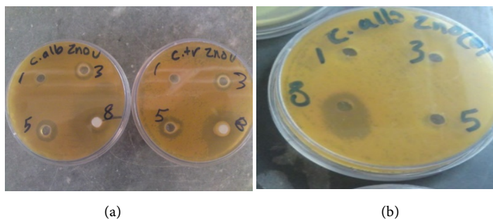
Figure 10. The best result of well method for (a) sample 3 (ZnO391) and (b) sample 4 (ZnO45) pictures showing inhibition zone on C. tropicalis (20, 15 mm) and C. albicans (20, 20 mm) in order with highest concentration 80 \mu gr/ml.
