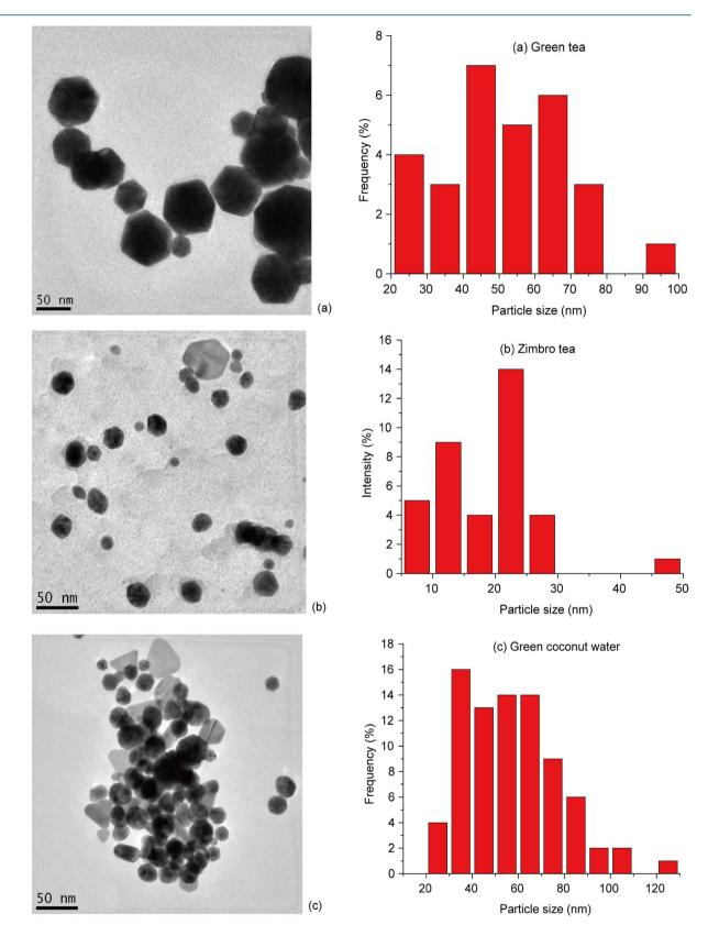
**Figure 4.** TEM micrographs and particle size distribution histograms of AuNPs reduced and stabilized with (a) Green tea, (b) Zimbro tea and (c) Green coconut water.
