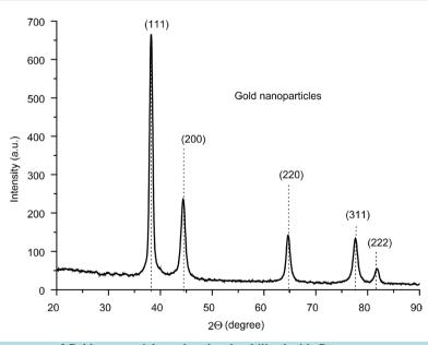
Figure 2. X-ray diffractograms of Gold nanoparticles reduced and stabilized with Green tea.
