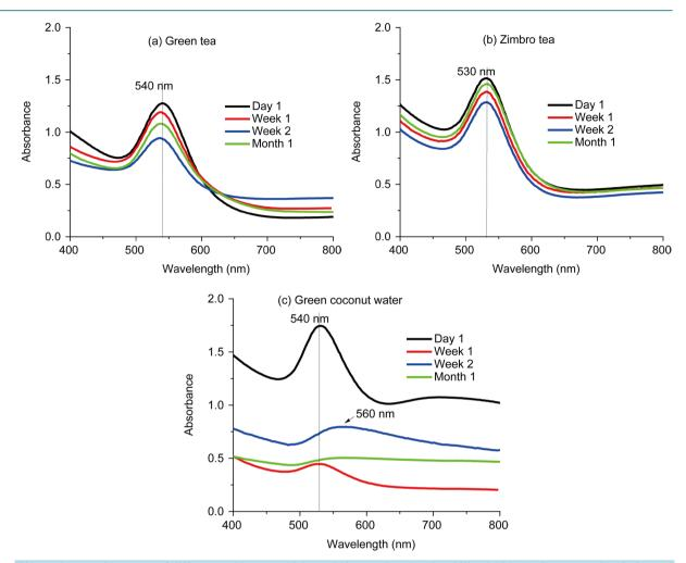
Figure 1. UV-Vis spectra of different gold nanoparticles solutions reduced and stabilized with (a) Green tea, (b) Zimbro tea and (c) Green coconut water at 25°C.
