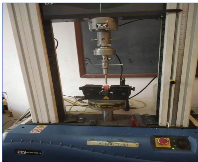
[Table/Fig-8]: Analysis of fracture resistance under compressive load using universal testing machine.
