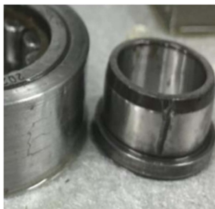
Figure 23. Inner ring fault bearing.
