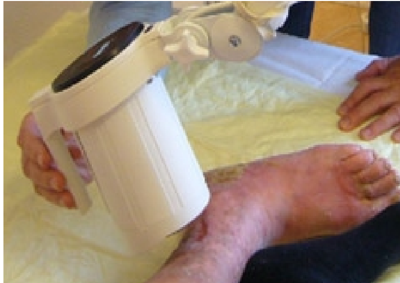
Fig. 2. The W-200 device for wireless micro-electrostimulation applications
