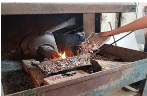
Fig. 5. Plastic Coating of Aggregate
