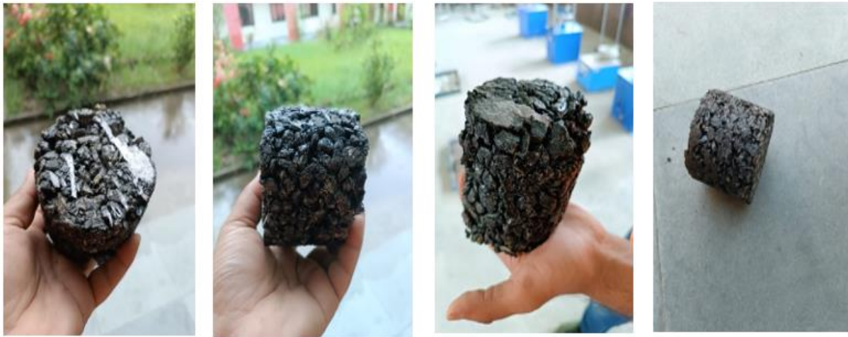
Fig. 7.8%,10%,12%, and 14% plastic mixes samples (from left)
