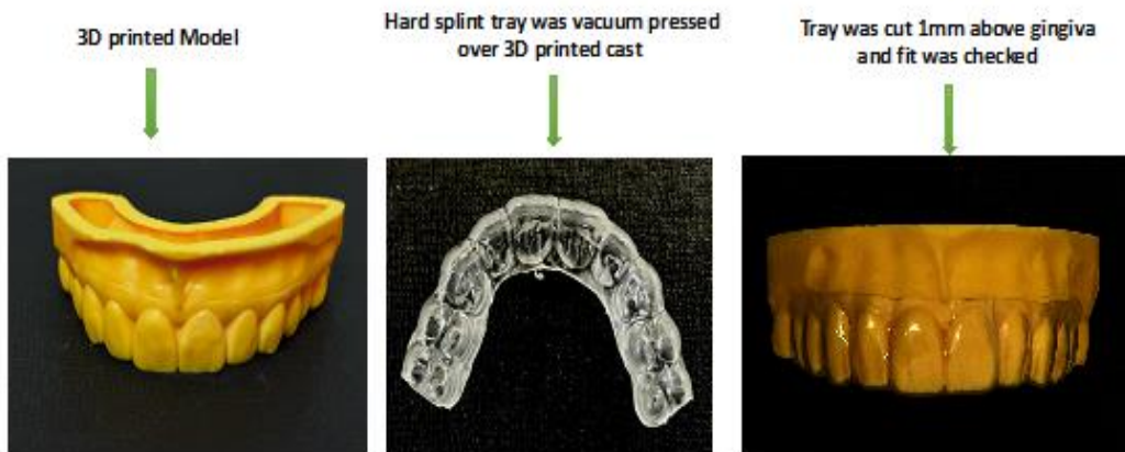
Fig. 3. Shows 3D printed model, hard splint tray, fit of the tray was check on 3D printed model and cut 1mm above the gingiva
