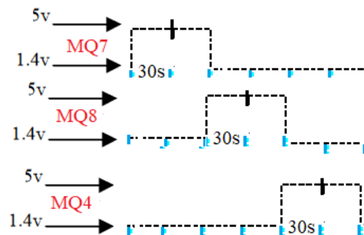
Fig. 8. Heating 3 MQ sensors with only a single one at 5V and the two others at 1.4V
