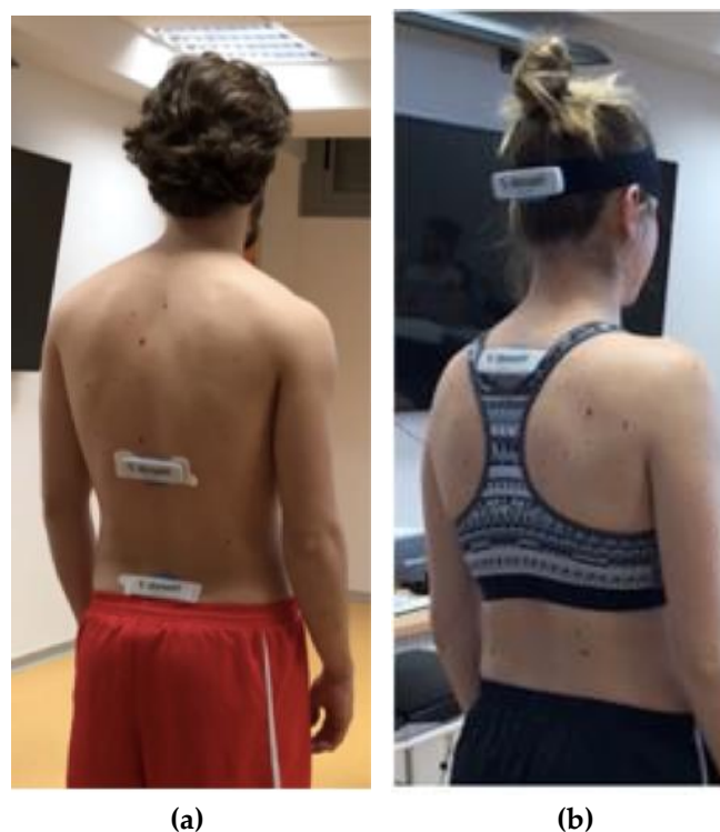
Figure 2. Range of motion (ROM) assessment with inertial motion units (IMUs). (a) Lumbar assessment. Subject position and device location. (b) Cervical assessment. Subject position and device location.
